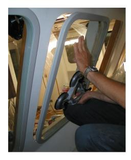
Once the window is centered, press firmly on the window until all sides are flat against the bulkhead.
